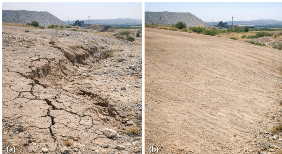
Fig. 2. Visual comparison of the technogenic deposit surface condition: (a) untreated area characterized by cracking and erosion features; (b) conserved area after six months of monitoring, demonstrating improved surface integrity, absence of visible cracks, and enhanced stability.
