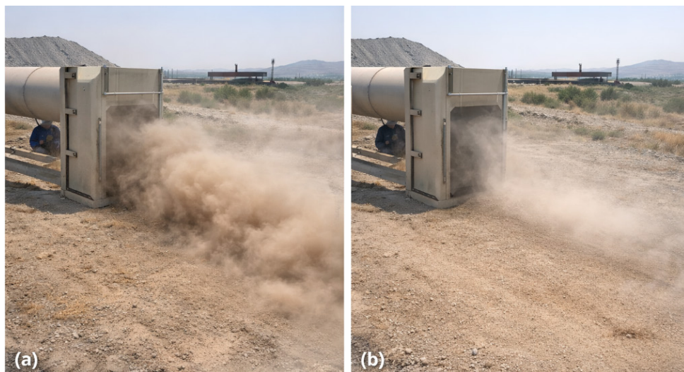
Fig. 1. Results of wind erosion simulation for the technogenic deposit: (a) untreated surface under airflow of 12–15 m/s, demonstrating intensive dust emission and material loss; (b) conserved surface after compaction and protective layer installation, showing significantly reduced dust generation and improved resistance to wind erosion.
